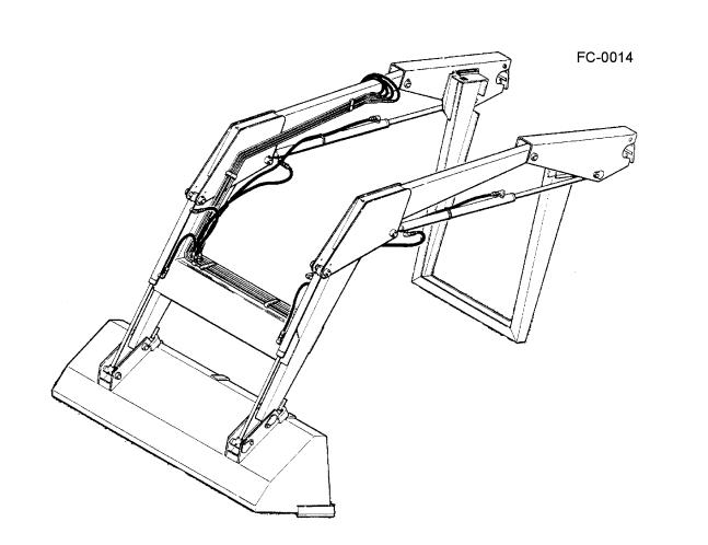
The Bush Hog 2647 Loader is designed for two and four-wheel drive tractors. They are intended to lift only loose materials that will fit in the bucket. All cylinders are double-acting. Parking stands support loader so tractor can be "driven in" for quick attaching.
